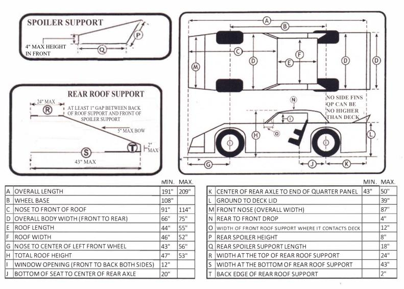
A maximum of 3 spoiler supports are allowed. Spoiler supports must all be the same length and a maximum of 9" tall. Rear Roof Supports must be the same length on both sides. It is OK to have one rear Roof Support open and one closed. Rear Roof Supports must not extend past the rear end of the roof. (Must start to angle down at the rear end of the roof) Roof must be straight at the front and back (90 degrees to the sides of the car) Roof may be flat or curved. No lip allowed on the rear of roof.
